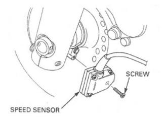
2. Remove the screw and speed sensor from the speedometer gear.
