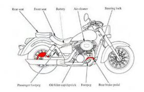
The rear brake on the ACE is a more simple Drum-style brake. In normal use, this brake only provides about 25% of the stopping power. Anymore and the rear wheel would lock up. It is also the brake most often used when the bike is standing still at a light, for example. It is inspected for wear at the drum, pedal height and free play and the stop light switch actuation point.
