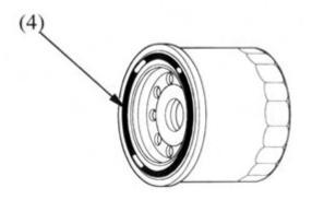
Apply a thin coat of oil to the new oil filter rubber seal (4). Install the new filter and snug it up **BY HAND**. The torque is only supposed to be 7 ft.lbs. and you can easily do this just with your hands. Use a rag if your hands are too greasy for a good grip.
