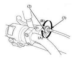
For minor adjustments, adjust the free play at the lever end as follows...
