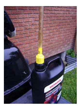
I use one of these type of funnels that can attach directly to a jug and has a nice flexible hose on the end and a shut off built in.
