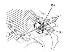
If the adjustment can't be reached at the lever end, then adjust it further from the clutch end as follows...
