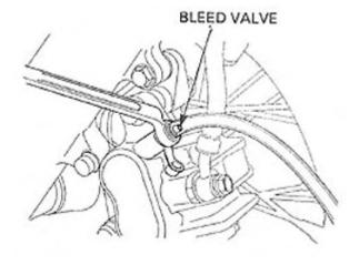
Connect a tube to the Bleed Valve and put the other end in a clean container.
