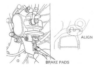
Remove the pad pin and the brake pads.
