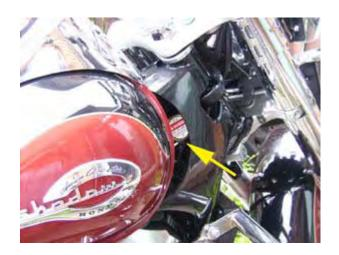
While the service manual asks you to remove the gas tank, you really only need to pull it aft a few inches, so you can access the radiator cap. Remove the seats and the tank mounting bolt and pull the tank back a few inches. Just be careful with the fuel line on the left hand side. With the tank back a few inches, you can easily remove the one clip on the neck cover and access the radiator cap (see arrow). Remove the radiator cap now.
