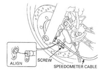
7. Install the speedometer cable and tighten the screw securely.
