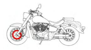
The front brake wear is measured at the pads on the brake unit itself, and they should be checked at each regular maintenance interval.
