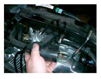
I also removed the forward cylinder ignition coil from the frame and moved it and the two plug wires back and out of the way... to give a bit more access room above the cylinders.
