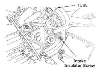
Disconnect the sub-air cleaner tube from the front side carburetor.
