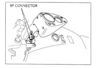
Remove the speedometer by removing the four hex-head bolts. Lift the assembly up and disconnect the 9-pin connector. Now is a good time to clean under there!
