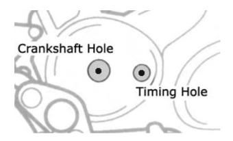
Remove the caps from the crankcase hole and the timing hole on the left-side crankcase cover.
