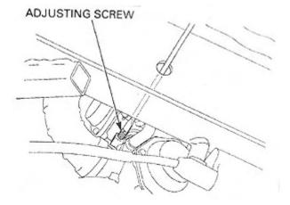
Note: The base carburetor is the REAR carb. (No.1)
