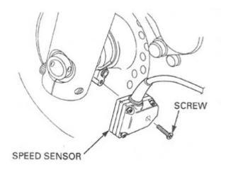
8. Install the speed sensor and tighten the screw securely.
