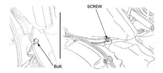
Remove the two (2) air cleaner housing bolts (not the 6 hex head bolts for the cover!). Then loosen the air cleaner housing to chamber band clamp with the screw. Pull the air cleaner housing away.
