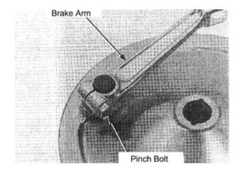
Install the brake arm on the brake cam, aligning the punch marks on the arm with those on the cam. Install and tighten the pinch bolt to **22 ft.lb. (3.0 kgf.m)**.
