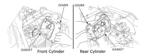
Remove the cylinder head covers and gaskets. Take care not to damage the gaskets or to scratch the clear coat finish on the covers. You might also have to remove the coolant lines to get the covers out. If you do, watch that you don't spill coolant onto the heads and in the oil. Take it slow and careful here!
