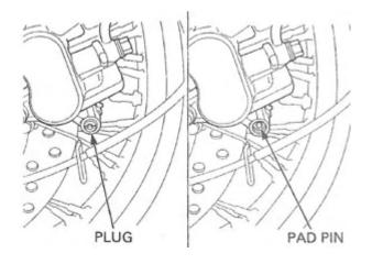
Remove the pad pin plug and loosen the pad pin under the plug.
