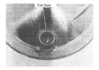
Remove the Felt Seal.
