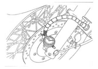
Check the brake disc for warpage using a dial indicator while rotating the front wheel.
