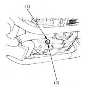
First warm the oil up by taking your bike for a short ride. To drain the oil, remove the oil filler cap/dipstick (#5 on bottom picture), the crankcase drain plug (1) and the gasket(2). Make sure to drain the oil in an approved container and dispose of it properly.
