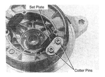
Install the Set Plate and NEW Cotter Pins.
