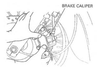
Push the caliper pistons all the way in by pushing the caliper body inward to allow for installation of new brake pads.
