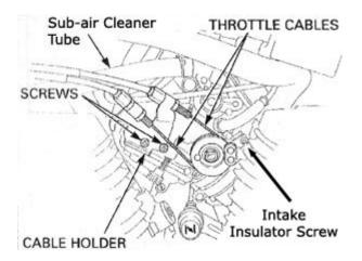
Remove the screws and throttle cable holder.
