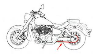
The service life of the drive chain is dependent upon proper lubrication and adjustment. Poor maintenance can cause premature wear or damage to the drive chain and sprockets. The drive chain should be inspected prior to every day's riding, adjusted for slack when required and lubricated every 800km or following any riding done in rain.
