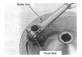
Remove the Pinch Bolt and Brake Arm.
