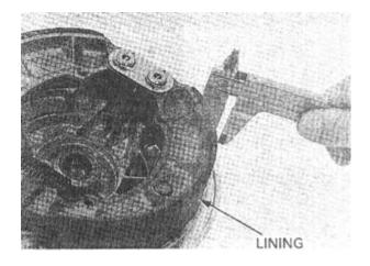
Measure the brake lining thickness.
