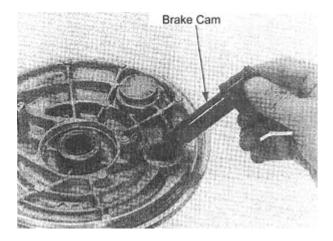
Remove the Brake Cam.
