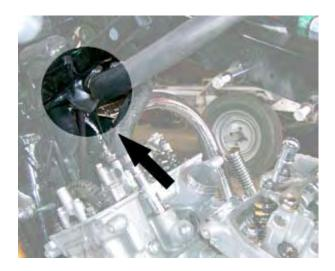
Remove the mounting bolt holding the thermostat housing and move the housing upward to give you room to remove the cylinder head covers.
