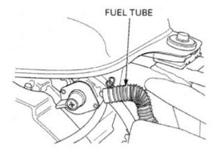
Place a rag under the fuel valve to catch any fuel that comes out then remove the fuel tube from the valve by squeezing the clip ends and sliding the clip back down the tube. Pull the tube from the valve. On the other side of the tank there is a slim air vent tube that you can just pull off the tank easily. Remove the fuel tank mounting bolt and then slide the tank back a bit and lift it clear of the bike. Make sure the speedometer harness is out of the clip holder on top.
