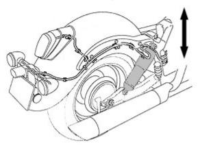
Check the action of the shock absorbers by compressing them several times. Check the entire shock absorber assembly for signs of leaks, damage or loose fasteners. Replace damaged components which cannot be repaired and tighten all nuts and bolts.
