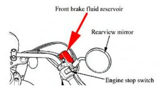
The Brake fluid level should be checked before every day's ride and during every maintenance cycle. The fluid should be changed every 2 years or at 19,200 km (12,000 miles), whichever comes first. The recommended brake fluid is **Honda DOT 4**.
