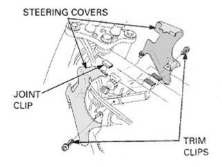
Remove the trim clips, then remove the two halves as an assembly. Remove the joint clip if you wish to separate the halves.
