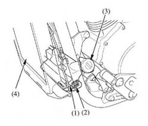
The reserve tank is located behind the radiator(4). Check the coolant level in the reserve tank while the engine is at normal operating temperature. It should be between the UPPER(1) and the LOWER(2) level marks. When the coolant level is at the LOWER mark, then add new coolant up to the UPPER mark. **Always** add coolant to the reserve tank only. Do not attempt to open the radiator cap while the engine is hot.
