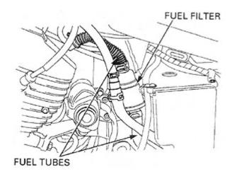
Remove the left-side cover. Check the fuel lines for deterioration, damage or leakage. Replace the fuel lines if necessary.
