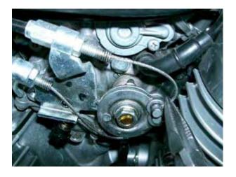
Remove the throttle cables from the throttle link.
