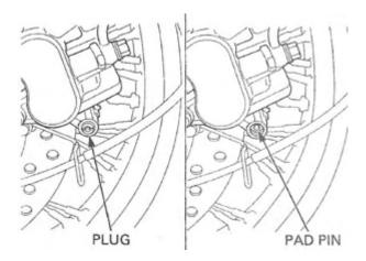
Install the pad pin by pushing the pads against the pad springs to align the pad pin holes and the pin holes in the pads and the caliper.
