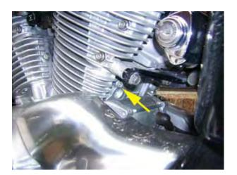
Remove the drain plug on the rear cylinder (see arrow). There's really no way to catch this fluid and it will just drain over your engine, so wash it up after. Luckily, there is very little fluid that comes from this drain. Also, when you open this drain port up, this will release an air lock and let more fluid drain out the water pump. Let things drain for a few minutes and then put both drain plugs back in and torque the bolts to 9 lbf-ft. It is also advisable to use new sealing washers.
