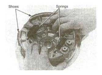
Remove the Brake Shoes and Springs.
