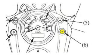
To check the safety cut-out feature, sit on the bike and turn the ignition on. With the side stand down, the side stand light (6) on the tank gauge cluster should be illuminated. Move the side stand up and the light should go out.
