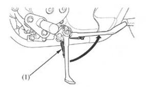
Sit on the bike and keep it vertical. Check the side stand for proper movement and for return spring tension. A broken or damaged spring (1) can allow the side stand to drop while riding, causing it to scrape and causing the engine to quit.
