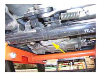
Put your container under the water pump and remove the drain plug, which is located on the bottom of the engine, left side, below the kick stand (see arrow). You are draining not only the front cylinder, but also the radiator and the big hoses, so there's almost 2 liters that comes out here. Leave the plug out for now.
