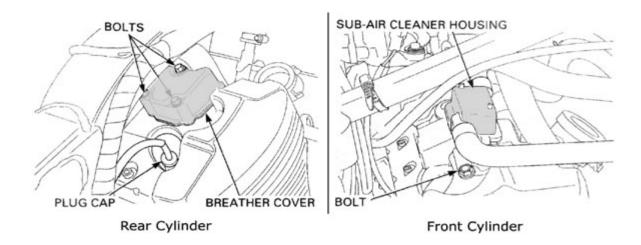
Remove the sub-air cleaner housings from both cylinders. The rear cylinder is only held on with one bolt and the front cylinder's is held on with 3 bolts.
