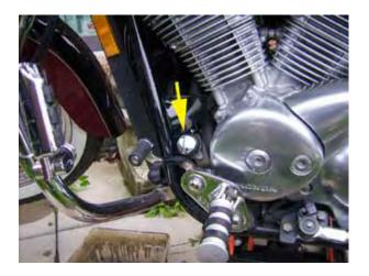
Remove the cap from the coolant reservoir.
