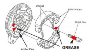
Apply grease to the brake shoe-to-cam contact surfaces.
