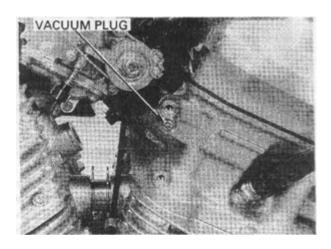
Remove the vacuum plugs and washers from the cylinder head intake ports.
