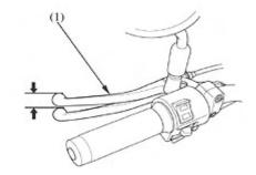
Clutch Adjustment may be required if the motorcycle stalls when shifting into gear or tends to creep; or if the clutch slips, causing the engine to race ahead when accelerating hard or climbing steep hills. Free play at the lever (1) should be kept between 10-20mm (0.4-0.8in).
