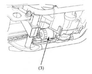
Remove the oil filter (3) with a filter wrench or by hand and let the remaining oil drain out. Discard the oil filter.
