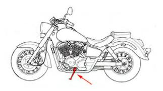
The ACE is equipped with a side stand only, on the left side of the bike. It only needs to be checked for damage or loss of return spring tension and for the safety cut-out switch proper operation.
