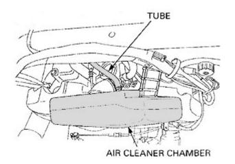
For the air chamber, you need to loosen the band clamps at the intakes for the carburetors. Then pull the chamber a little ways from the frame and disconnect the crankcase breather tube from the chamber. Remove the air chamber.
