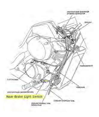
Check the brake light switch operation and adjustment by applying the brakes with the ignition turned on. Operation of either the front brake lever or the rear brake pedal should illuminate the rear brake light.
