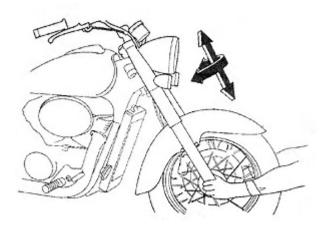
Support the motorcycle securely and raise the front wheel off the ground. Check that the handlebar moves freely from side to side. If the handlebar moves unevenly, binds or has vertical play, then inspect the steering head bearings
