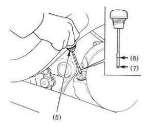
Check the condition of the oil plug gasket(2) and re-use if it's ok. Replace it every other oil change or any time it looks worn. Fill the crankcase with the new oil until it reads on the dipstick(5) and then secure the cap. **Apx.**
